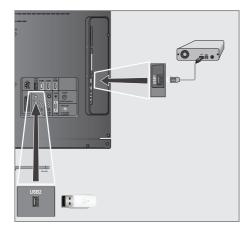
Connect the »USB2 (HDD)« socket of the television and the corresponding socket of the data medium (external hard disk) using a USB cable:
